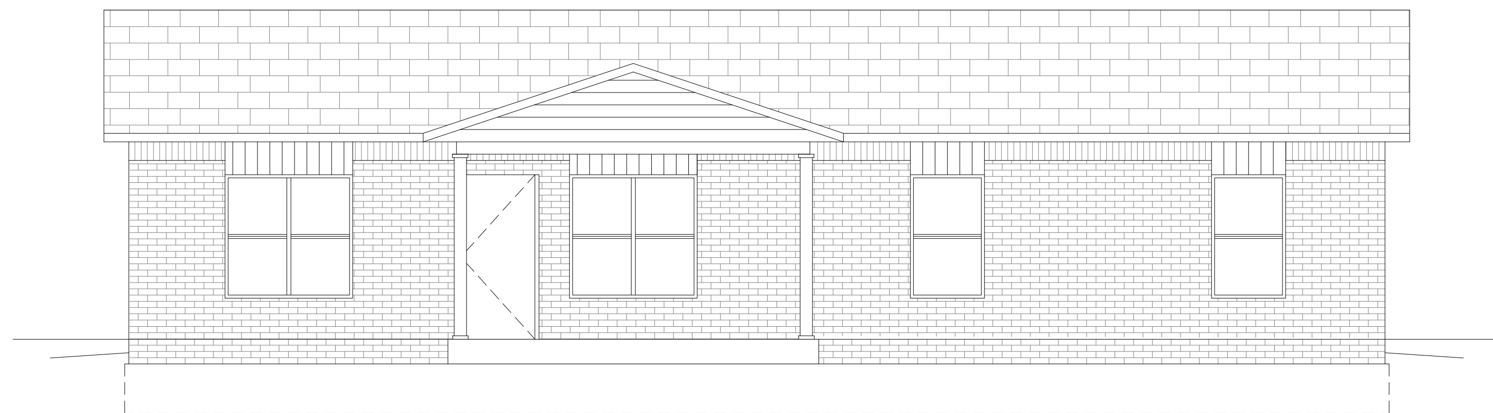
B 4 Bedroom Front Elevation Scale: 1/4" = 1'-0"
