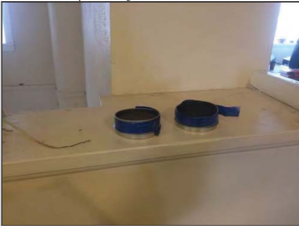
Photo 2: Radon canisters placed within the 2 nd floor lobby of the Cherokee Nation Capital Building.
