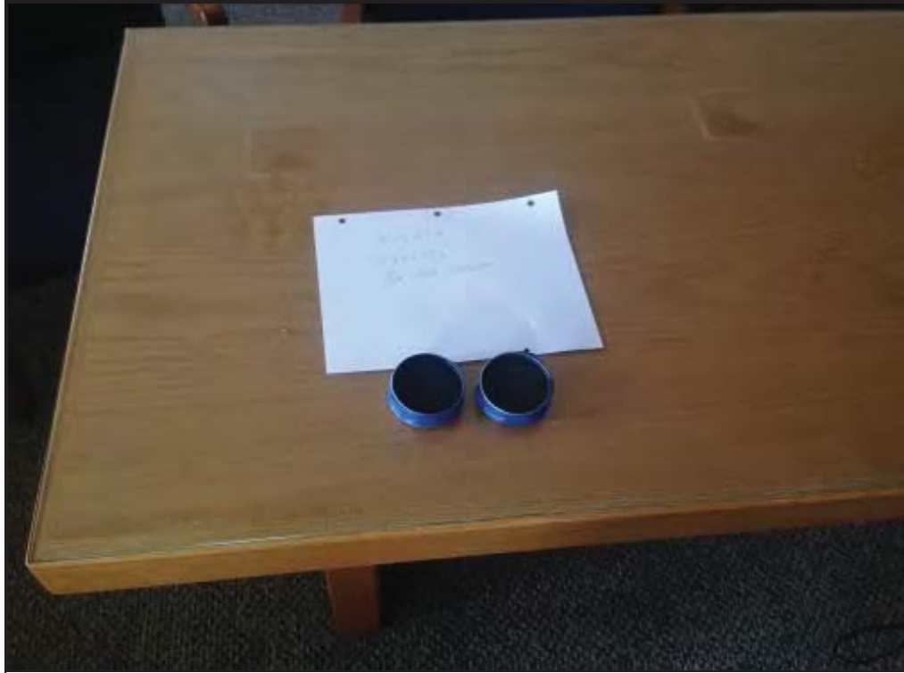
Photo 1: Radon canisters placed within the 2 nd floor courtroom of the Cherokee Nation Capital Building.
