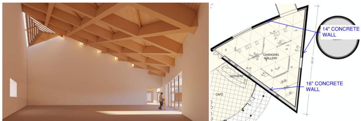
Figure 6-10 Changing Gallery – Interior Architectural Axonometric (L) and Architectural Plan (R)
