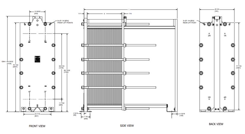
PACK LENGTH MAX (A): 35.18 Inch FIXED THICKNESS (TF): 3.25 Inch OVERALL LENGTH (L): 80.14 Inch MOVABLE THICKNESS (TM):2.25 Inch
