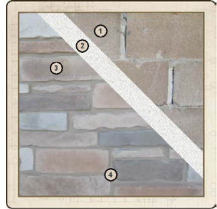
① Unpainted masonry or concrete, ② mortar setting bed, ③ manufactured stone, ④ mortar joint.
