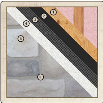
① Rigid backwall (sheathing, in this example), ② weather-resistant barrier, ③ metal lath, ④ mortar setting bed, ⑤ manufactured stone, ⑥ mortar joint.
