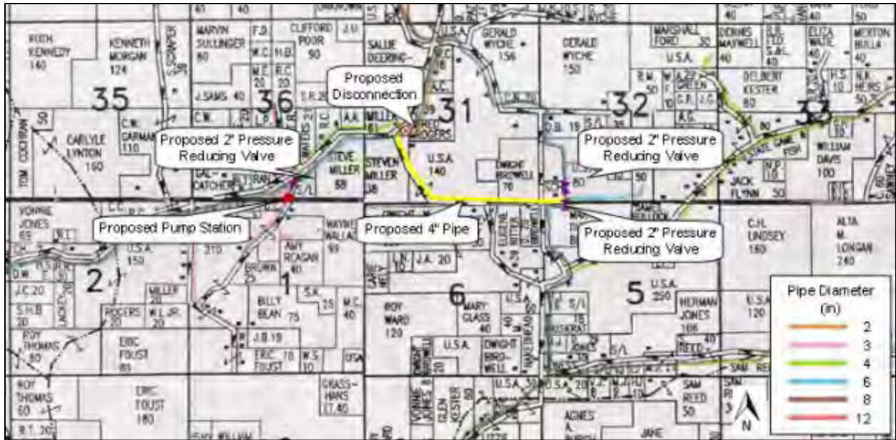
Figure 20: Approximate location of three pressure reducing valves, 5,100-ft of additional pipe (shown in yellow), and disconnection proposed in the Bell area.
