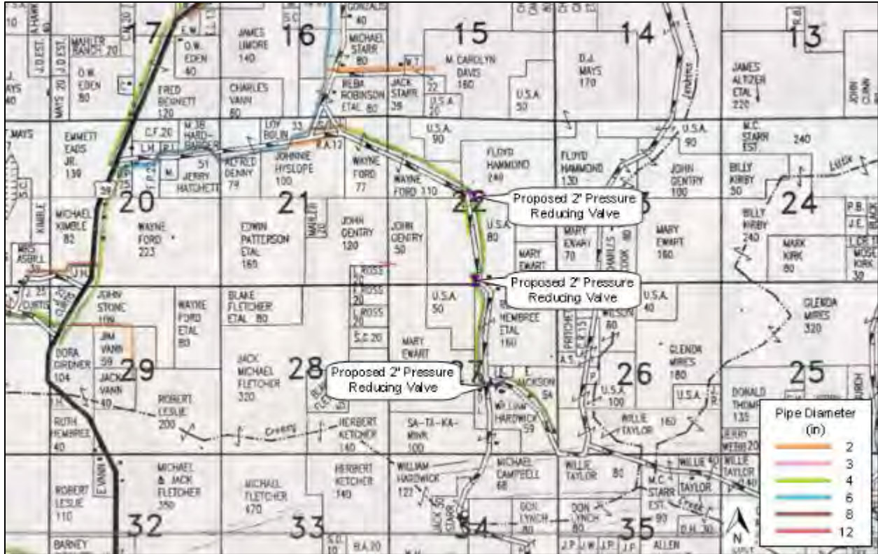
Figure 18: Approximate location of three pressure reducing valves proposed in the Killer Mountain area.
