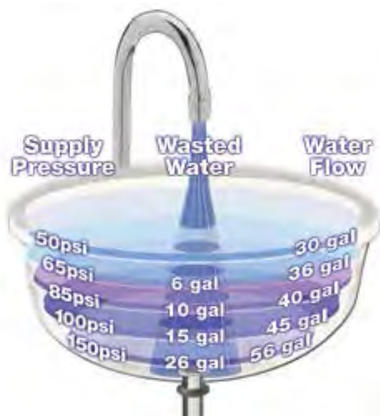
Figure 22: Conceptual illustration of water use at higher pressures and flows increases wasted water for the same amount of use ( http://www.watts.com/pages/learnAbout/reducingValves.asp?catId=64 ).
