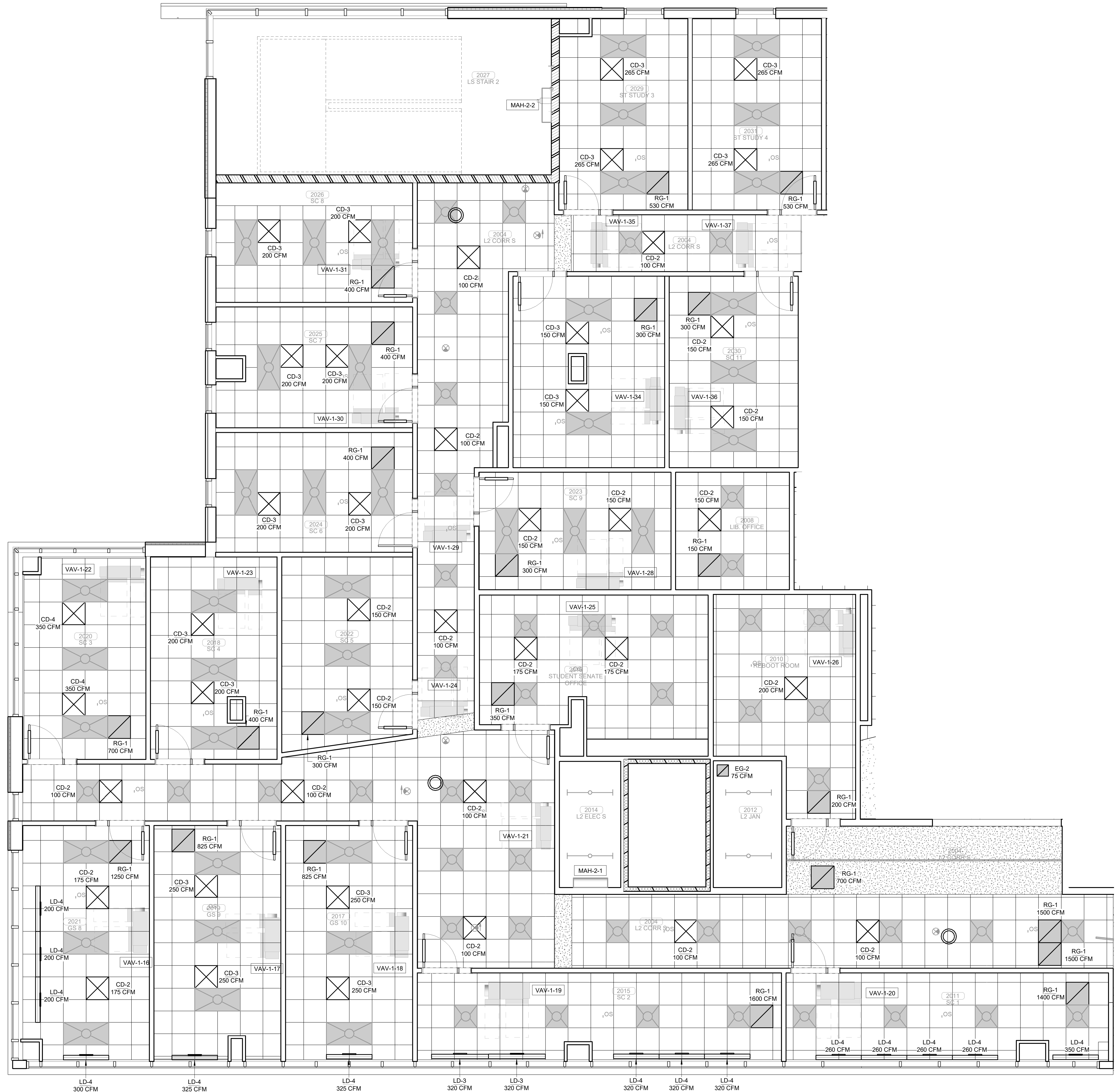
1 ENLARGED MECHANICAL REFLECTED CEILING PLAN LEVEL 02 1/4" = 1'-0"
