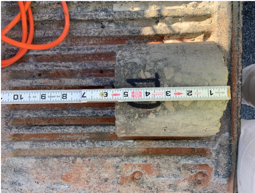
Fig. 2 – C-1 Core Sample 5 1/2" Asphalt Depth
