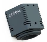
The M A517HD1080 Series high definition camera outputs HDMI video at true 1080p HD resolution. The 1/3" C-mount design offers a compact and lightweight HD video solution. The on-camera push-button is used for one-push white balance and push-hold for image flip. Use with camera adapter M A528STHDC.
