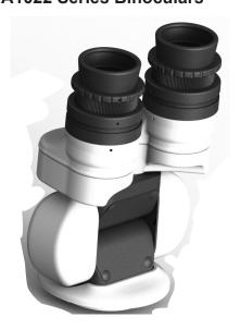
The inclinable binoculars allow for 0-220 degrees of tilt articulation. This feature accommodates multiple user heights while maintaining optimal ergonomic posture. It also allows the user to maintain this posture while moving the microscope head.
