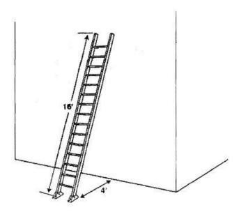
Portable ladders must be used at such a pitch that the horizontal distance from the top support to the foot of the ladder is about one-quarter of the working length of the ladder.
